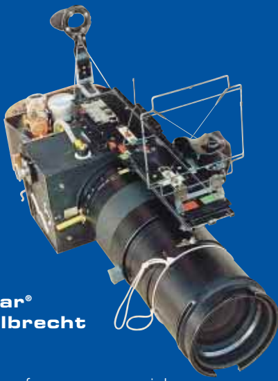
Fig. 3: Brugger's automatic aerial camera with a magazine for 30 m of unperforated 70-mm film which is flattened by vacuum against the pressure plate. The camera in this photo is fitted with a special 300 mm Planar® f/4 lens from Carl Zeiss.
